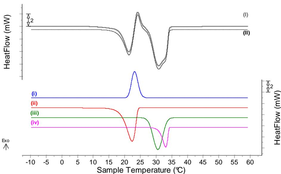
Figure 2 – Typical cocoa butter thermogram and associated peak separation
