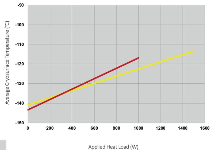
Single-circuit models; 25- 28°C cooling water; temperature shown is average of inlet and outlet temperature using typical cryocoil size; temperature difference between inlet and outlet at maximum load is typically 20°C; end point of each curve is maximum load for that model; performance at 50Hz can be 3- 5°C warmer than 60Hz performance shown.
