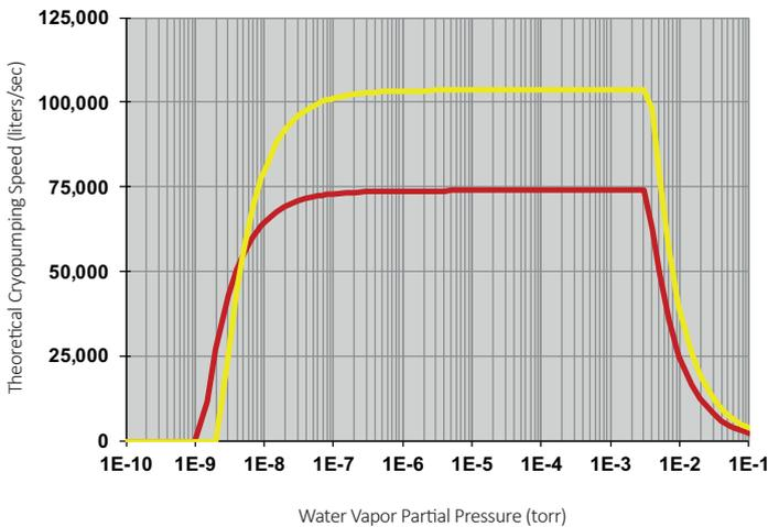
Single-circuit models; 25- 28°C cooling water; 2.4m refrigerant line; advertised cryocoil surface areas only; larger cryocoils will give greater pumping speeds and can be used in some applications; 25°C temperature in line of sight with cryocoil; 60Hz.
