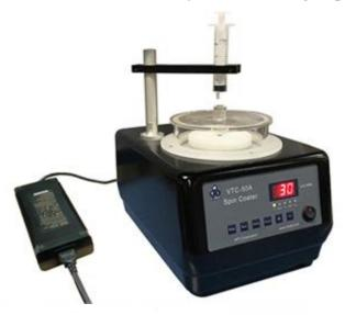
VTC-50A is an economic question Spin Coater with a vacuumless chunk that is designed for the quality coating of sol-gel at the lowest cost. By using grooved spinning templates to hold samples on the rotating plate, the instrument provides the advantages of cost-effectiveness and ease of maintenance. Complete accessories are included for immediate use.
